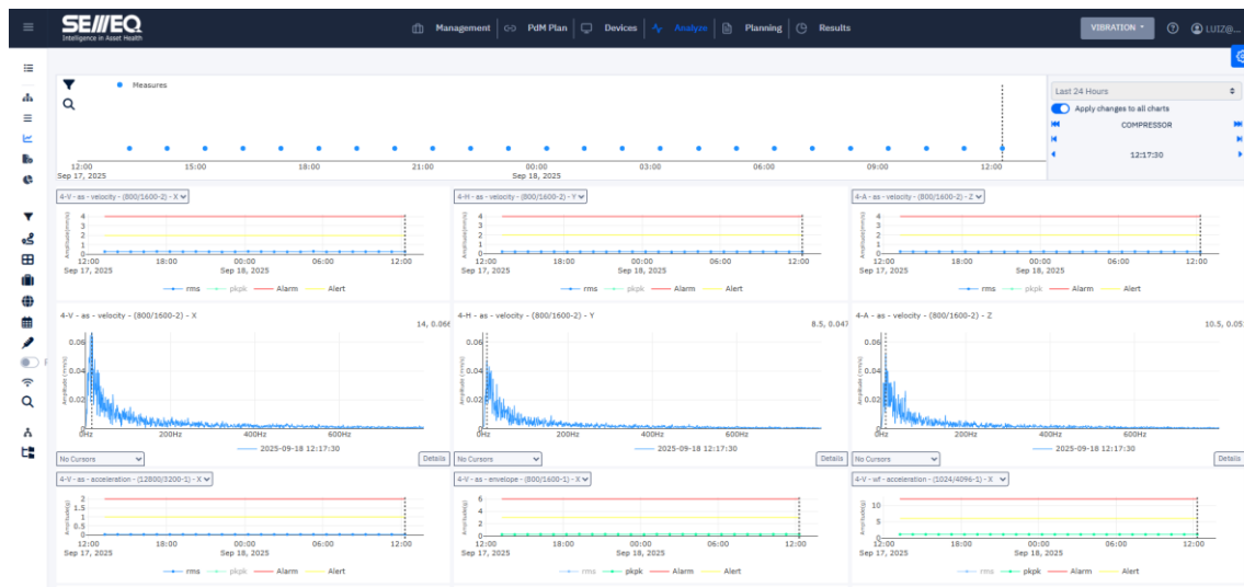
Figure 2 — Vibration Analysis dashboard from SEMEQ Portal Stream.
